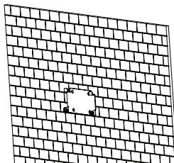
4. Align the rear notch of charger with the wall-mounted bracket and fit the screw holes of the right and left side. Tighten two wing nut screws by hand.
