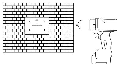
3. Use 4 Hexagonal Expansion Screws to secure the wall-mounted bracket (Use anti-theft hexagonal expansion screws) on the wall. Then level the bracket.
