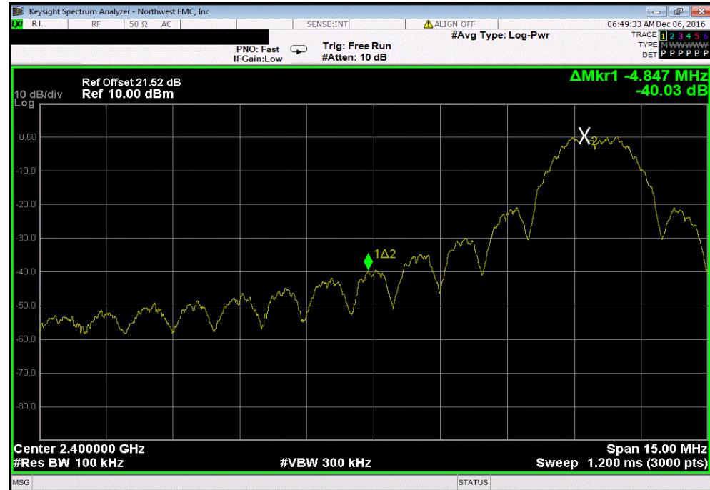
2400 MHz - 2483.5 MHz Band, OQPSK, High Ch, 2480 MHz
