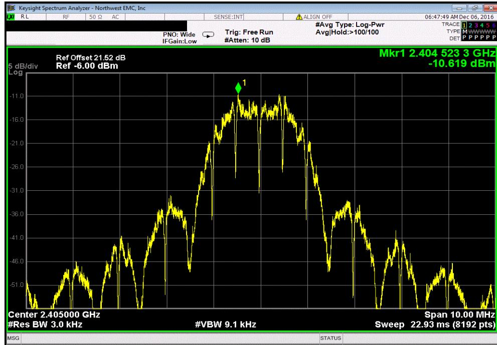
2400 MHz - 2483.5 MHz Band, OQPSK, Mid Ch, 2440 MHz
