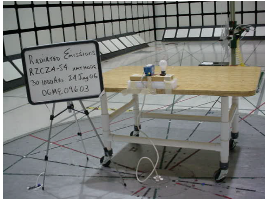
Radiated Emissions 30-1000MHz Test Set Up
