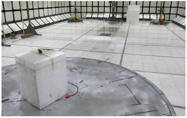
Radiated Measurement Setup 1GHz-25GHz
