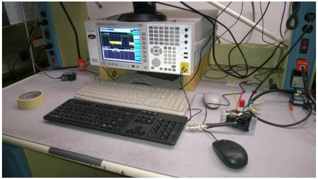
RADIATED MEASUREMENT SETUP 9kHz - 30MHz
