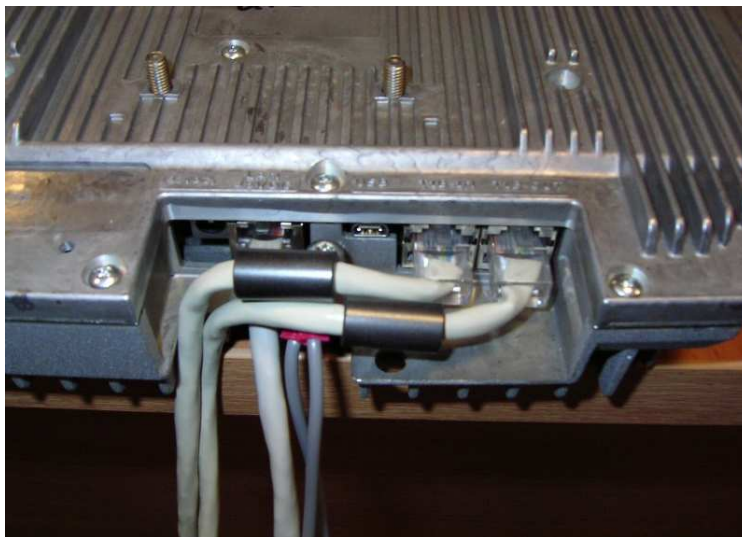
Figure 8 - Ethernet and TIB cabling
