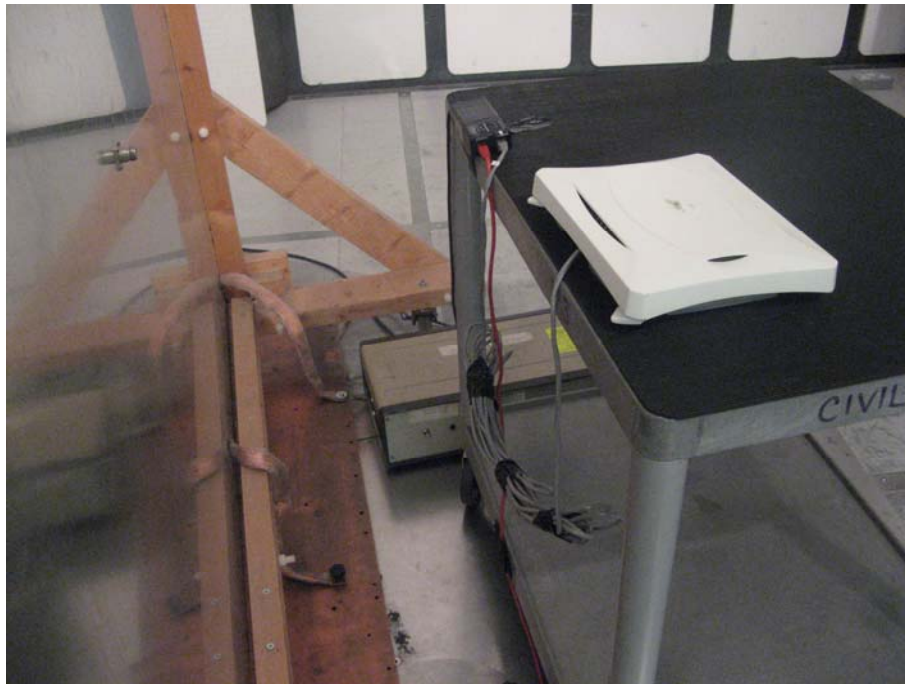
Conducted Emissions AC Power Port Test Setup
