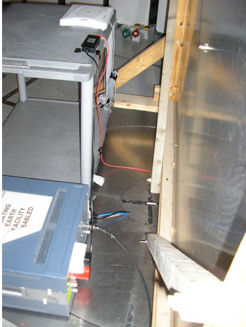
Conducted Emissions AC Power Port Test Setup
