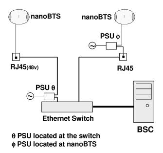
When using the ip.access model 126A Ethernet Switch and Power Inserter, external PSU's are not required, the NanoBTS is connected locally or via site cabling to the powered ports of the 126.
