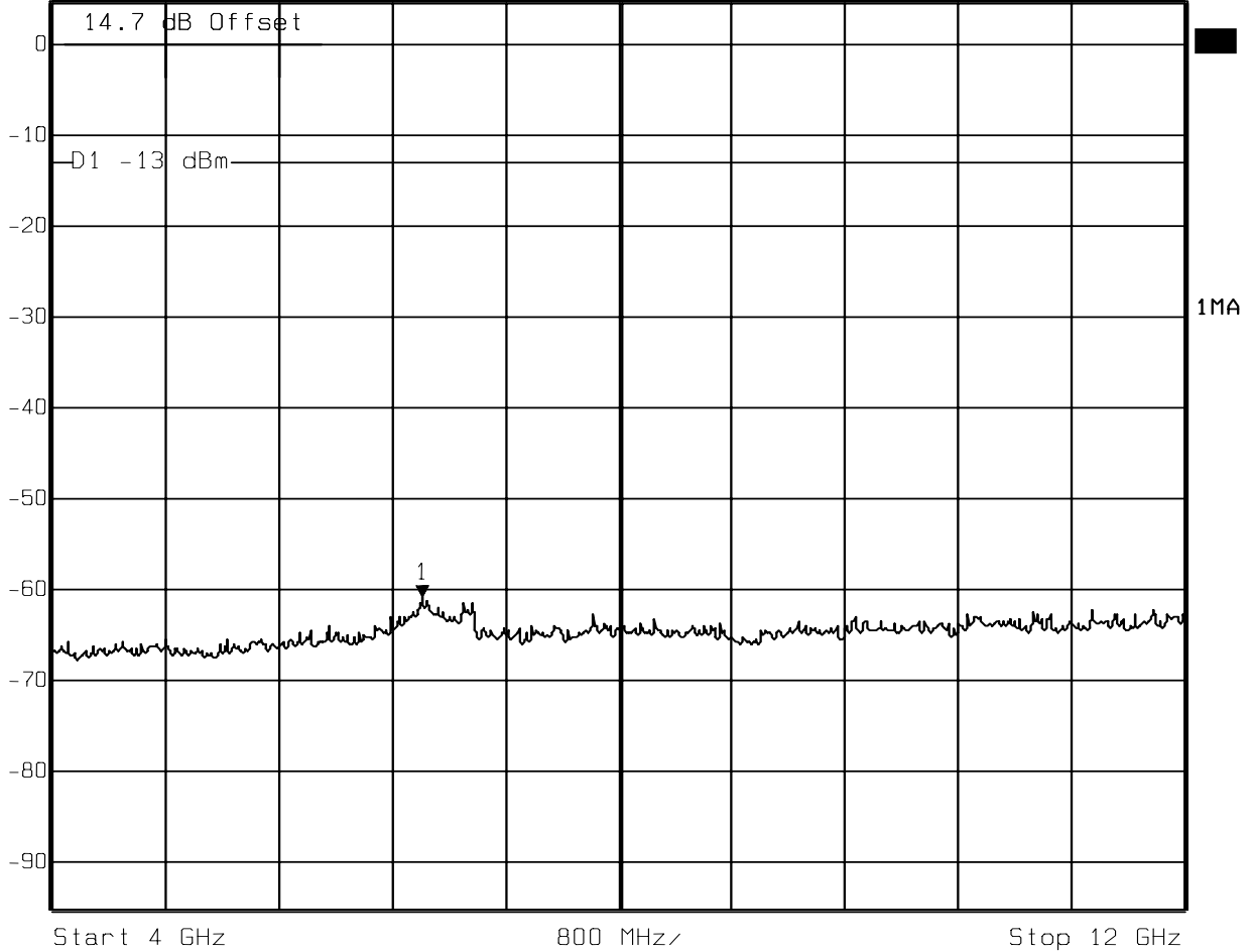
Spurious Emissions (4GHz - 12GHz) EDGE Mode Channel 661 (1960.0MHz) - Maximum Power
