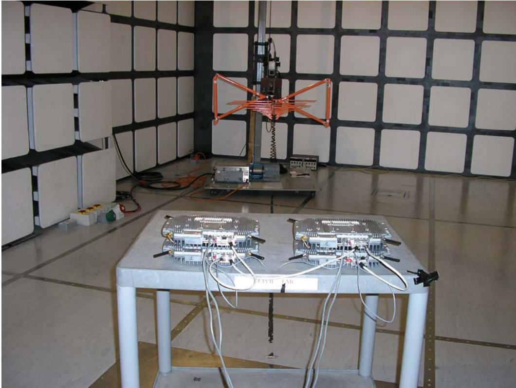
Radiated Emissions Test Set up
