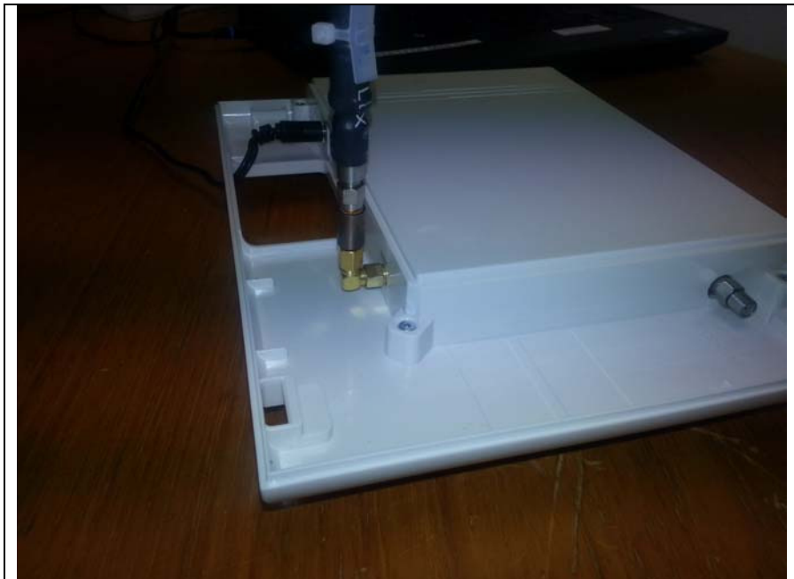
Fig 2 Test setup Conducted Emissions on Antenna port
