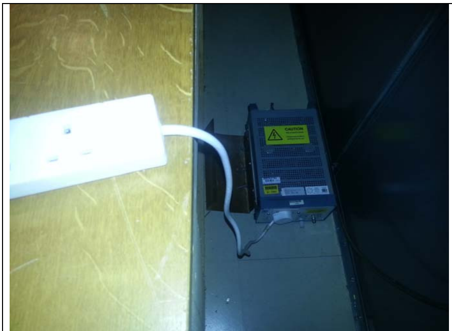
Fig 9 Test setup Conducted Emissions on the mains
