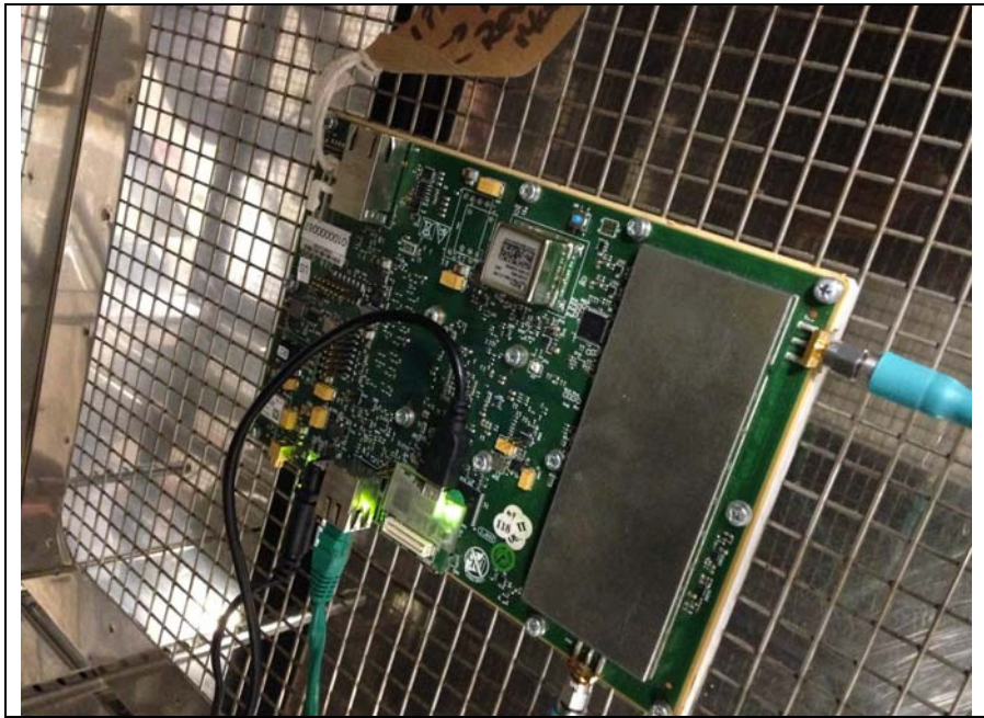
Fig 10 Test setup Temperature testing
