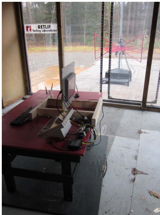
Horizontal Antenna Polarization, 30 MHz to 1 GHz
