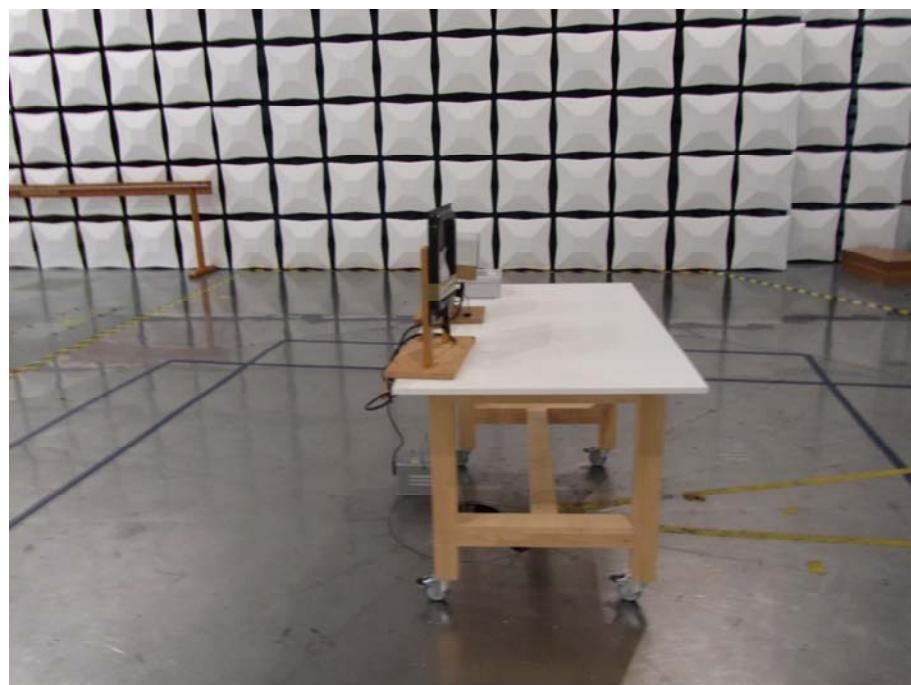
**Test setup for radiated emission measurement
