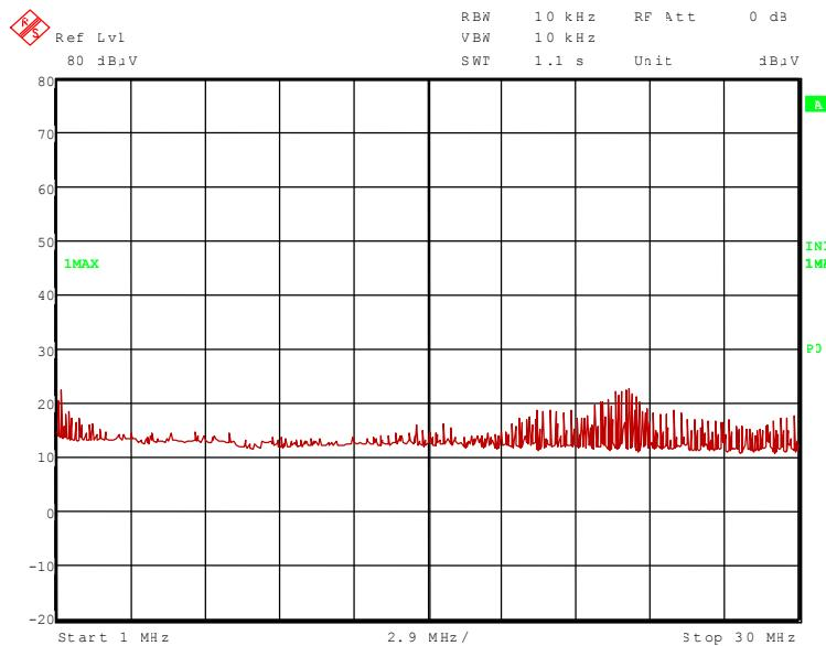
The following emissions were found according to FCC 47 CFR Part 15 section 15.209 (a).
