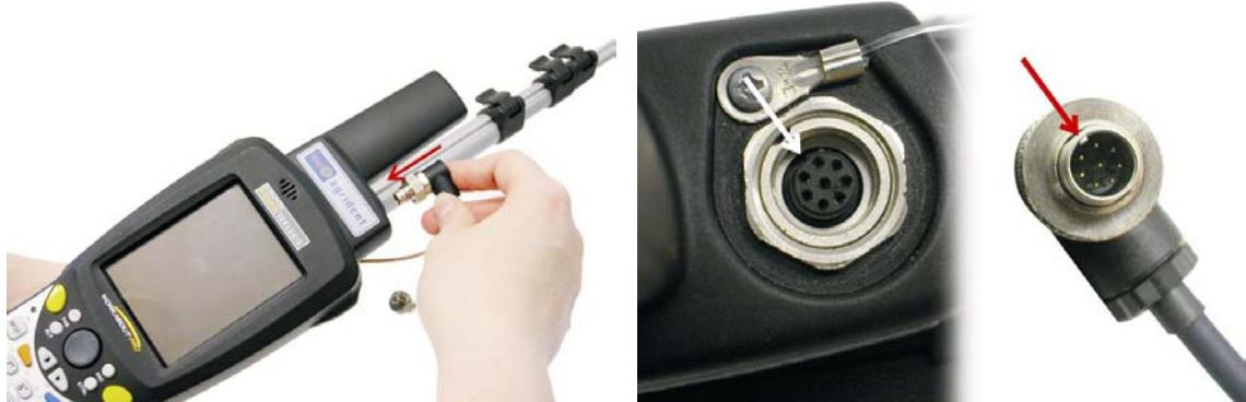
5. Put the Binder plug of the telescope antenna in the socket of the AIR200 reader.
