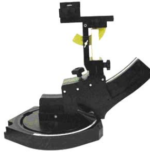
Device holder supplied by SPEAG
