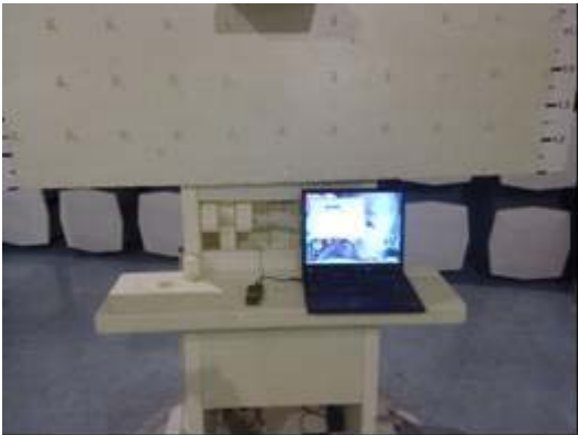
Picture 2. FCC Part 15B Radiated emissions
