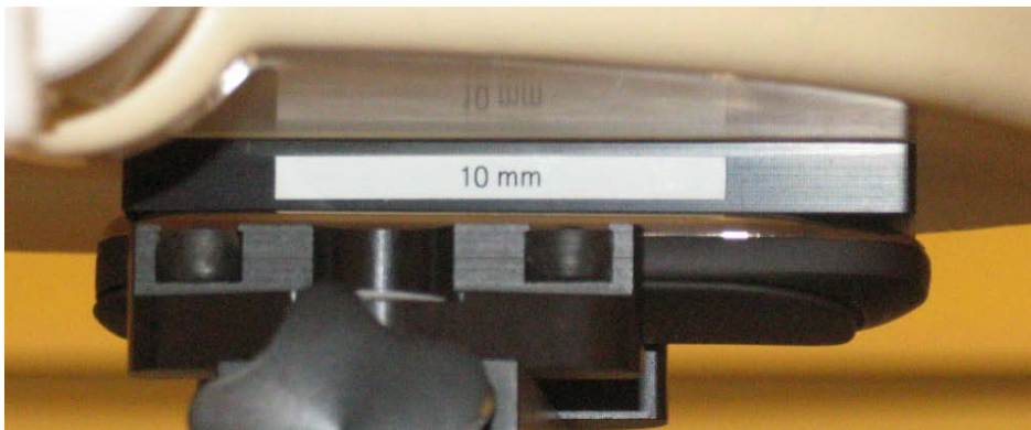
Photo of the device positioned for WR mode measurement – display facing phantom. The spacer was removed before the start of the measurements.
