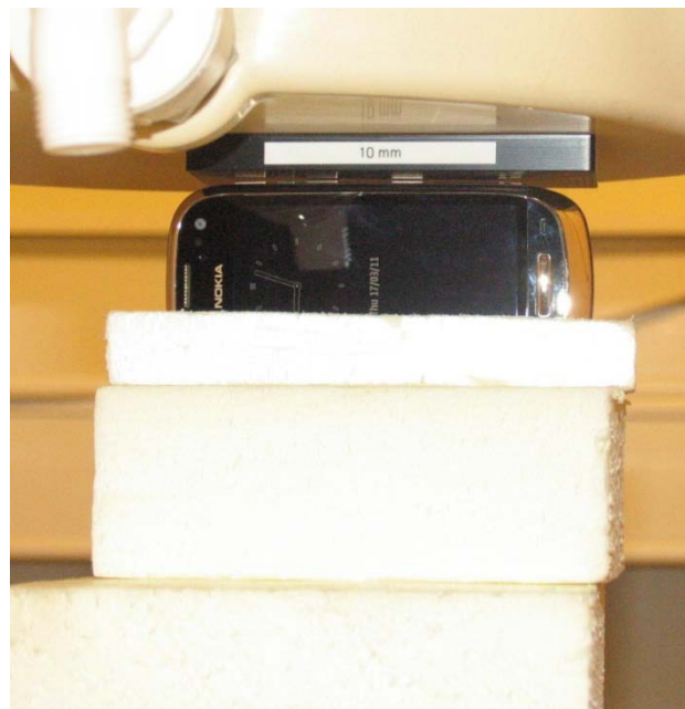
Photo of the device positioned for WR mode measurement – right edge facing phantom. The spacer was removed before the start of the measurements.
