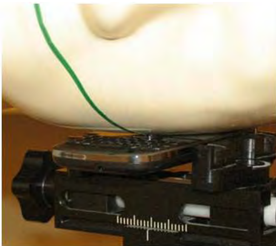
Photo of the Device in "cheek" position
