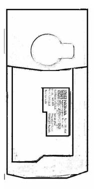
Rear view of phone with rear lid removed showing label position in battery compartment.
