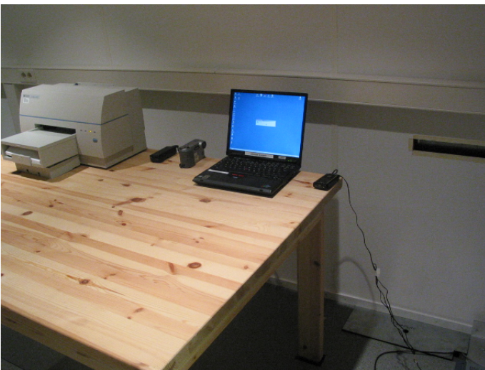
Picture 4 AC powerline conducted emission measurement GSM RX/Bluetooth TX + Computer peripherals
