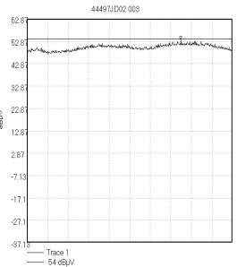
Start 6.0 GHz; Stop 8.0 GHz Ref 62.87 dBμV; Ref Offset 20.0 dB; 10 dB/div RBW1.0 MHz; VBW 1.0 MHz; Att 0 dB; Swp 50.0 mS Peak 7.496667 GHz, 53.2 dBμV Display Line: 54 dBμV; 16/05/2003 11:44:13
