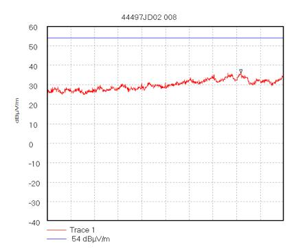
Start 18.0 GHz; Stop 26.5 GHz Ref 60 dBµV/m; Ref Offset 0.0 dB; 10 dB/div RBW 1.0 MHz; VBW 1.0 MHz; Att 0 dB; Swp 40.0 mS Peak 24.961 GHz, 35.91 dBµV/m Display Line: 54 dBµV/m; Transducer Factors: 18to26 17/04/2003 12:16:07
