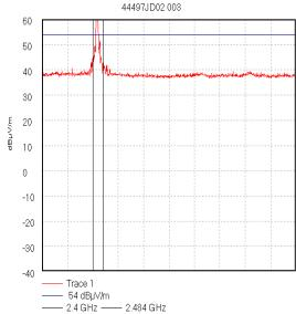
Start 2.0 GHz; Stop 4.0 GHz Ref 60 dBµV/m; Ref Offset 0.0 dB; 10 dB/div RBW 1000.0 kHz; VBW 1.0 MHz; Att 0 dB; Swp 20.0 mS Peak 2.431 GHz, 63.98 dBµV/m Display Line: 54 dBµV/m; ; Limit Test Failed Transducer Factors: 2 to 4 16/04/2003 16:26:52
