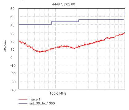
Start 30.0 MHz; Stop 1.0 GHz - Log Scale Ref 60 dBµV/m; Ref Offset 0.0 dB; 10 dB/div RBW 120.0 kHz; VBW 100.0 kHz; Att 0 dB; Swp 80.0 mS
