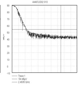
Start 2.479 GHz; Stop 2.485 GHz Ref 90 dBj\t/; Ref Offset 22.6 dB; 10 dB/div RBW 1.45 MHz; VBW 100.0 kHz; Att 0 dB; Swp 20.0 mS Peak 2.479007 GHz, 89.83 dBj\t/ Display Line: 54 dBj\t/; 27/05/2003 21:04:53
