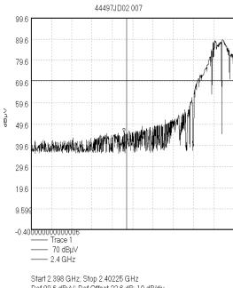
Start 2.398 GHz; Stop 2.40225 GHz Ref 99.6 dBjv/; Ref Offset 22.6 dB; 10 dB/div RBW 100.0 kHz; VBW 100.0 kHz; Att 0 dB; Swp 20.0 mS Marker 2.399946 GHz, 45.49 dBjv/ Display Line: 70 dBjv/; 27/05/2003 20:35:04
