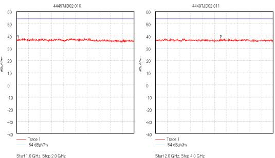
Start 1.0 GHz; Stop 2.0 GHz Ref 60 dBμ/Vm; Ref Offset 0.0 dB; 10 dB/div RBW 1000.0 kHz; VBW 1.0 MHz; Att 0 dB; Swp 20.0 mS Peak 1.016 GHz, 38.83 dBμ/Vm Display Line: 54 dBμ/Vm; Limit Test Passed Transducer Factors: 1 to 2 17/04/2003 16:43:25 Start 2.0 GHz; Stop 4.0 GHz Ref 60 dBμV/m; Ref Offset 0.0 dB; 10 dB/div RBW 1000.0 kHz; VBW 1.0 MHz; Att 0 dB; Swp 20.0 mS Peak 3.109 GHz, 38.37 dBμV/m Display Line: 54 dBμV/m; Limit Test Passed Transducer Factors: 2 to 4 17/04/2003 16:48:50
