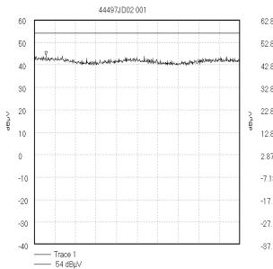
Start 4.0 GHz; Stop 6.0 GHz Ref 60 dBµV; Ref Offset 17.0 dB; 10 dB/div RBW 1.0 MHz; VBW 1.0 MHz; Att 0 dB; Swp 50.0 mS Peak 4.116667 GHz, 44.0 dBµV Display Line: 54 dBµV; 16/05/2003 11:32:15
