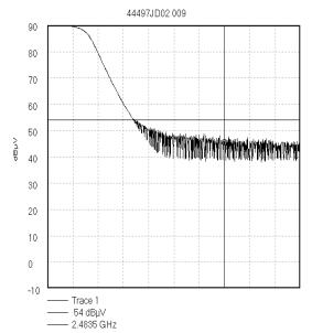
Start 2.48 GHz; Stop 2.485 GHz Ref 90 dBjtV; Ref Offset 27.0 dB; 10 dB/div RBW 1.45 MHz; VBW 100.0 kHz; Att 0 dB; Swp 20.0 mS Marker 2.4835 GHz, 44.8 dBjtV Display Line: 54 dBjtV; 27/05/2003 20:57:52
