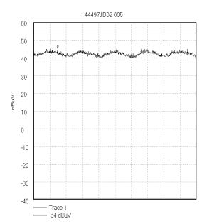
Start 8.0 GHz; Stop 12.5 GHz Ref 60 dBμV; Ref Offset 14.0 dB; 10 dB/div RBW1.0 MHz; VBW 1.0 MHz; Att 0 dB; Swp 90.0 mS Peak 8.6675 GHz, 45.17 dBμV Display Line: 54 dBμV; 16/05/2003 12:01:40
