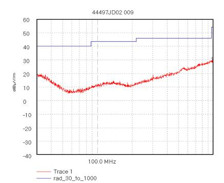
Start 30.0 MHz; Stop 1.0 GHz - Log Scale Ref 60 dBµV/m; Ref Offset 0.0 dB; 10 dB/div
