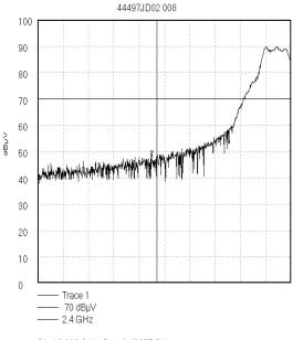
Start 2.398 GHz; Stop 2.40225 GHz Ref 100 dBµV; Ref Offset 27.0 dB; 10 dB/div RBW 100.0 kHz; VBW 100.0 kHz; Att 0 dB; Swp 20.0 mS Marker 2.399913 GHz, 48.38 dBµV Display Line: 70 dBµV; 27/05/2003 20:40:20
