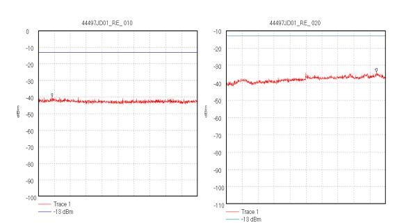
Start 2.0 GHz; Stop 4.0 GHz Ref 0 dBm; Ref Offset 10.0 dB; 10 dB/div RBW 1.0 MHz; VBW 1.0 MHz; Att 0 dB; Swp 20.0 mS Peak 2.173833 GHz, -40.04 dBm Display Line: -13 dBm; Transducer Factors: 2 to 4 30/04/2003 14:21:07
