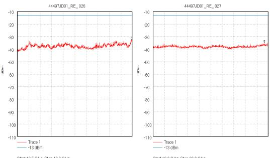
Start 12.5 GHz; Stop 18.0 GHz Ref -10 dBm; Ref Offset 10.0 dB; 10 dB/div RBW 1.0 MHz; VBW 1.0 MHz; Att 5 dB; Swp 40.0 mS Peak 17.957222 GHz, -32.8 dBm Display Line: -13 dBm; 02/05/2003 14:54:59 Start 18.0 GHz; Stop 20.0 GHz Ref -10 dBm; Ref Offset 10.0 dB; 10 dB/div RBW 1.0 MHz; VBW 1.0 MHz; Att 0 dB; Swp 20.0 mS Peak 19.931111 GHz, -35.08 dBm Display Line: -13 dBm; 02/05/2003 14:59:50
