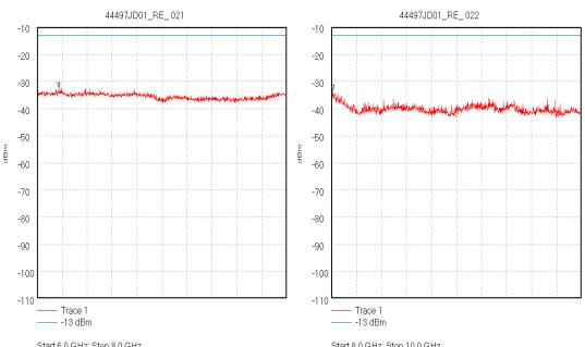
Start 6.0 GHz; Stop 8.0 GHz Ref -10 dBm; Ref Offset 10.0 dB; 10 dB/div RBW 1.0 MHz; VBW 1.0 MHz; Att 15 dB; Swp 20.0 mS Peak 6.173333 GHz, -32.32 dBm Display Line: -13 dBm; 02/05/2003 14:26:53 Start 8.0 GHz; Stop 10.0 GHz Ref -10 dBm; Ref Offset 10.0 dB; 10 dB/div RBW 1.0 MHz; VBW 1.0 MHz; Att 10 dB; Swp 20.0 mS Peak 8.011111 GHz, -33.15 dBm Display Line: -13 dBm; 02/05/2003 14:31:55
