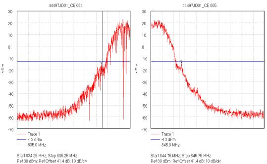
Start 834.25 MHz; Stop 835.25 MHz Ref 30 dBm; Ref Offset 41.4 dB; 10 dB/div RBW 2.068966 kHz; VBW 10.0 kHz; Att 0 dB; Swp 340.0 mS Marker 834.995556 MHz, -15.37 dBm Display Line: -13 dBm; ; Limit Test Failed 14/05/2003 19:38:04 Start 844.75 MHz; Stop 845.75 MHz Ref 30 dBm; Ref Offset 41.4 dB; 10 dB/div RBW 2.068966 kHz; VBW 10.0 kHz; Att 0 dB; Swp 340.0 mS Marker 845.021111 MHz, -13.98 dBm Display Line: -13 dBm; ; Limit Test Failed 14/05/2003 19:40:09
