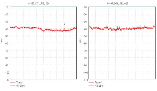
Start 6.0 GHz; Stop 8.0 GHz Ref-10 dBm; Ref Offset 10.0 dB; 10 dB/div RBW 1.0 MHz; VBW 1.0 MHz; Att 10 dB; Swp 20.0 mS Peak 7.642222 GHz, -35.52 dBm Display Line: -13 dBm; 02/05/2003 14:44:32 Start 8.0 GHz; Stop 12.5 GHz Ref -10 dBm; Ref Offset 10.0 dB; 10 dB/div RBW 1.0 MHz; VBW 1.0 MHz; Att 10 dB; Swp 20.0 mS Peak 8.0 GHz, -34.32 dBm Display Line: -13 dBm; 02/05/2003 14:48:32
