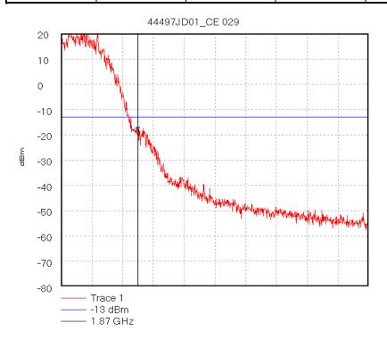
Start 1.86975 GHz; Stop 1.87075 GHz Ref 20 dBm; Ref Offset 42.8 dB; 10 dB/div RBW 3.0 kHz; VBW 10.0 kHz; Att 0 dB; Swp 340.0 mS Marker 1.870001 GHz, -18.8 dBm Display Line: -13 dBm; 14/05/2003 10:46:40
