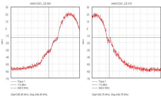
Start 845.95 MHz; Stop 846.95 MHz Ref 30 dBm; Ref Offset 41.4 dB; 10 dB/div RBW 2.068966 kHz; VBW 10.0 kHz; Att 0 dB; Swp 340.0 mS Marker 846.494444 MHz, -31.85 dBm Display Line: -13 dBm; ; Limit Test Failed 14/05/2003 20:14:35 Start 848.75 MHz; Stop 849.75 MHz Ref 30 dBm; Ref Offset 41.4 dB; 10 dB/div RBW 2.068966 kHz; VBW 10.0 kHz; Att 0 dB; Swp 340.0 mS Marker 849.01778 MHz, -15.22 dBm Display Line: -13 dBm; ; Limit Test Failed 14/05/2003 20:39.41
