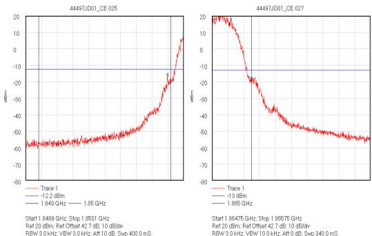
Start 1.8489 GHz; Stop 1.8501 GHz Ref 20 dBm; Ref Offset 42.7 dB; 10 dB/div RBW 3.0 kHz; VBW 3.0 kHz; Att 10 dB; Swp 400.0 mS Marker 1.849977 GHz, -16.94 dBm Display Line: -12.2 dBm; 12/05/2003 16:11:36
