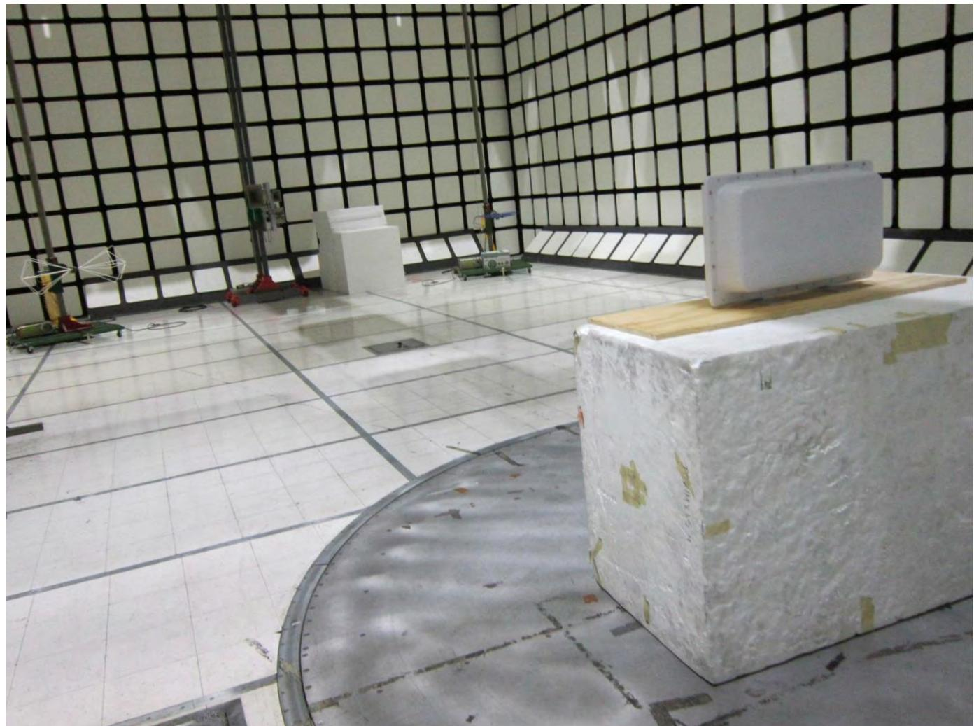
**Radiated Emissions Measurements above 1GHz**
