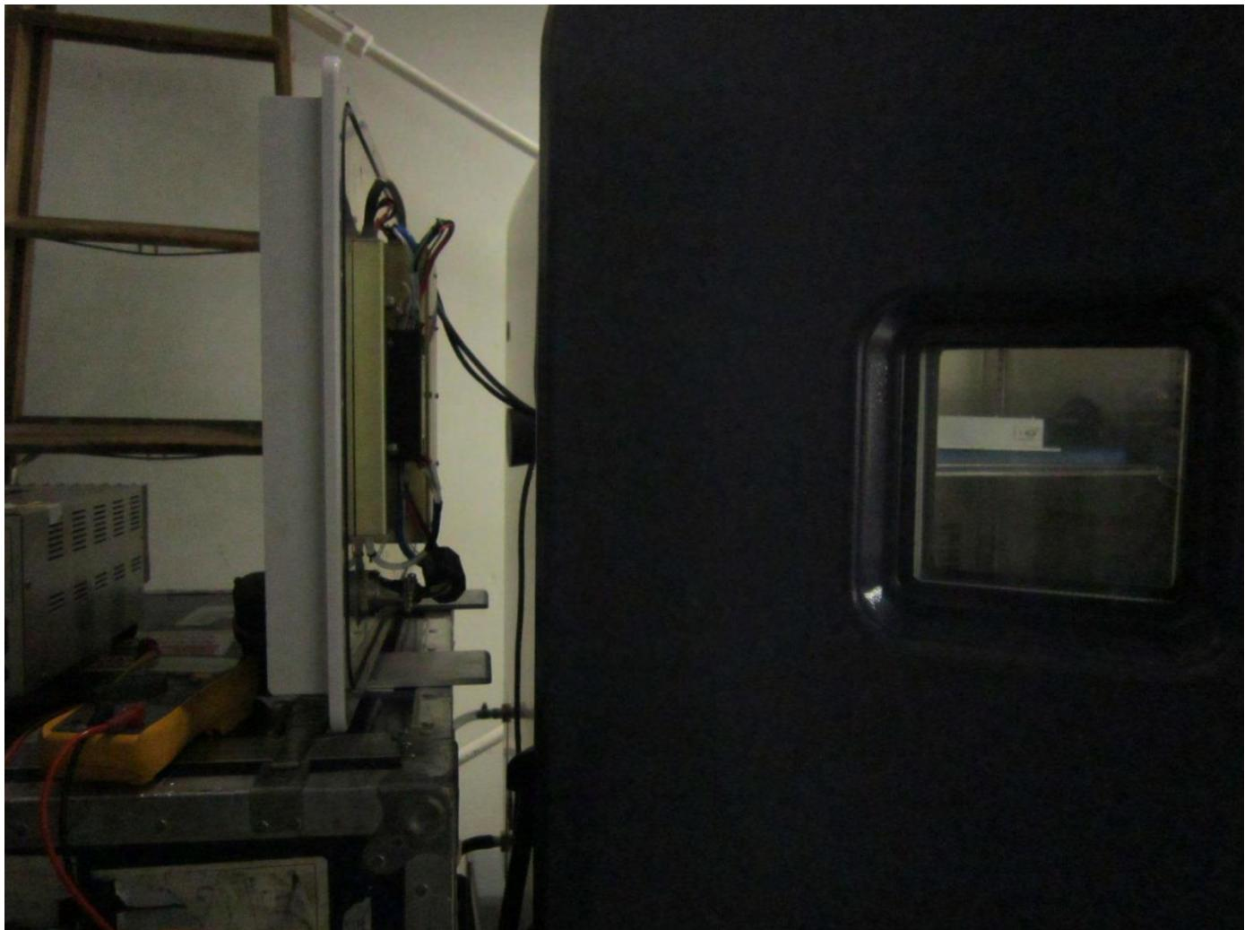
**Temperature Stability Measurements – essential part of transmitter inside the temperature chamber**
