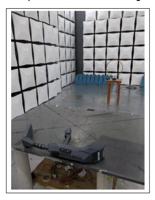
Radiated Spurious Emissions: Less than 30 MHz
