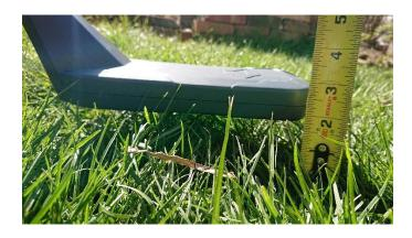
To set the antenna height, hold the unit as it would normally be used and adjust the pole extensions until the antenna face is flush against the ground, locking the pole extensions:
