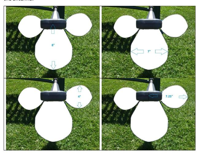
The antenna is intended to be held approximately 2" above the ground cover surface (soil, mulch, gravel) and is intended to detect tags that are buried up to 4" under the surface. The antenna should be kept parallel to ground surface to maximize the ability to detect the RFID tags that are buried parallel to the ground surface.
