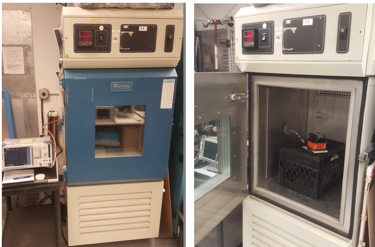
Figure 3.3 Frequency Tolerance Test Setup
