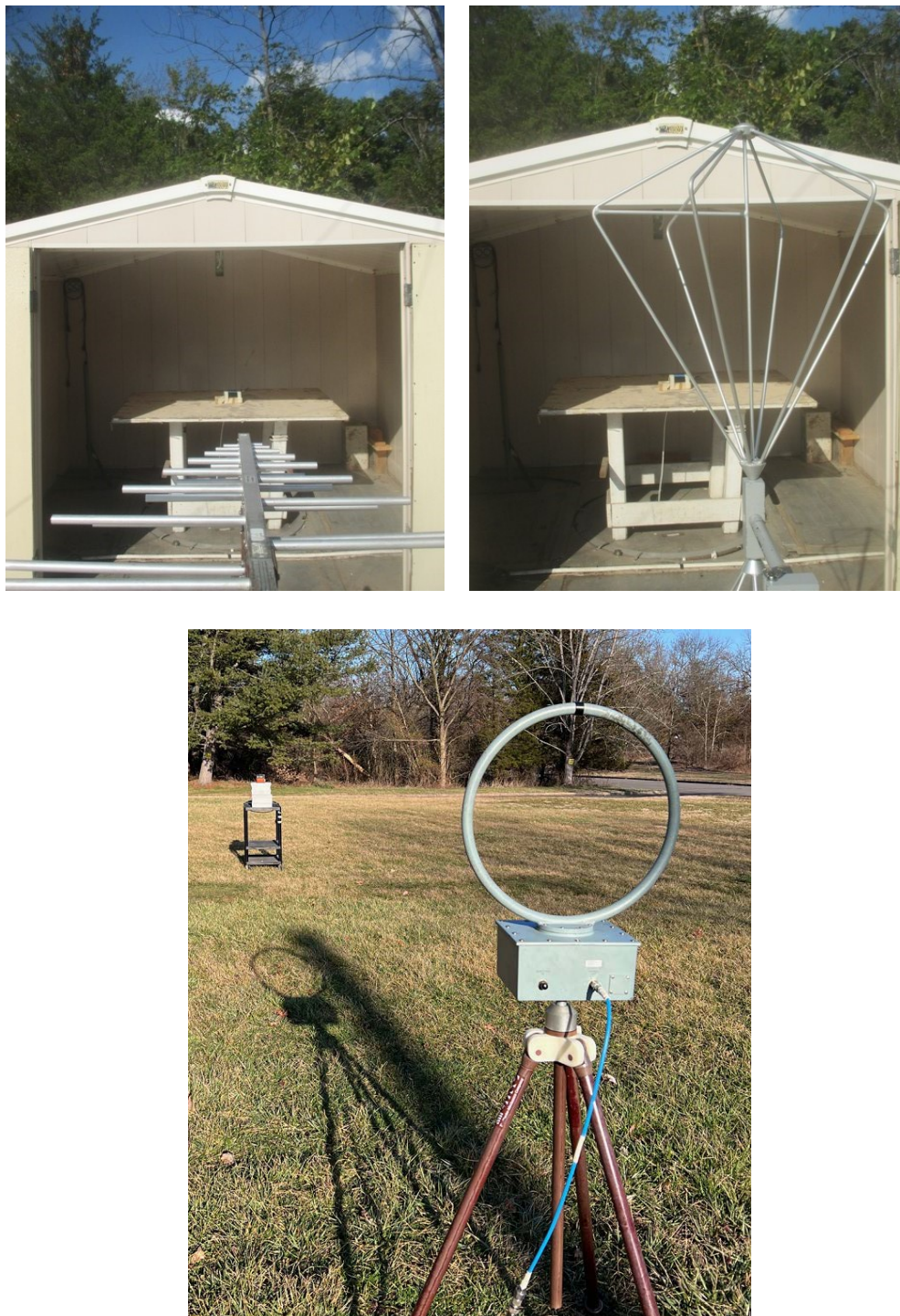
Figure 3.1 Radiated Emission Test Setup
