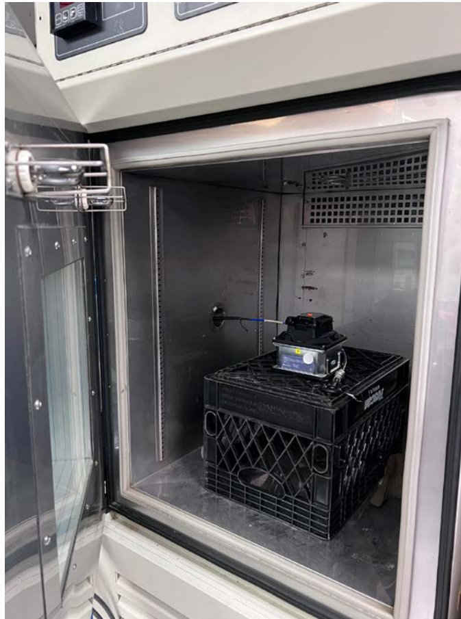
Figure 3.3 Frequency Tolerance Test Setup
