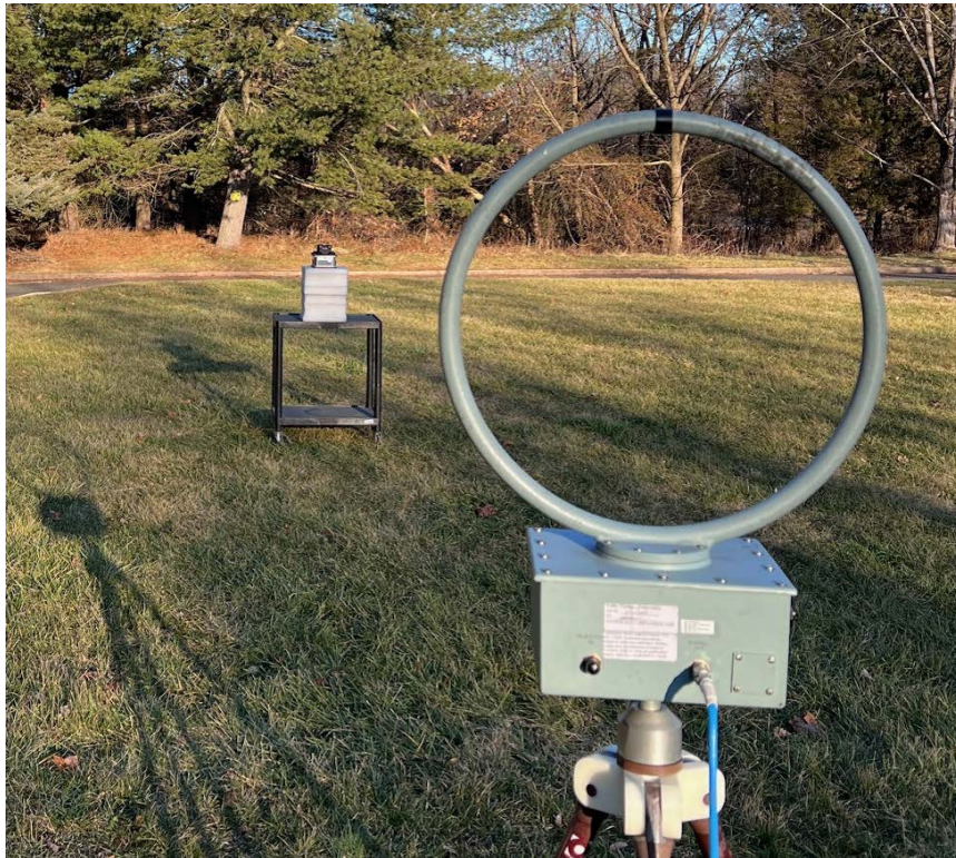
Figure 3.1 Radiated Emission Test Setup
