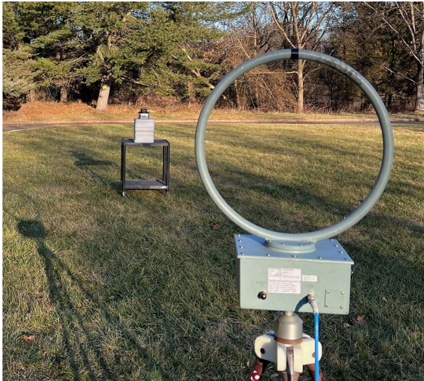
Figure 3.1 Radiated Emission Test Setup
