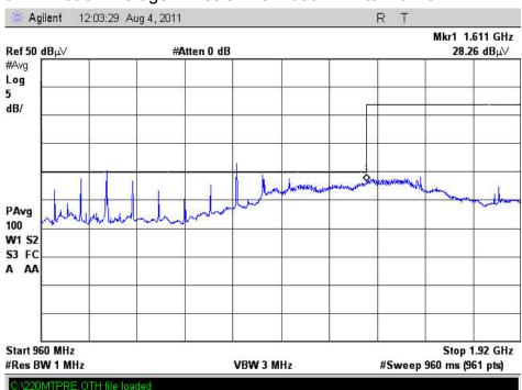
Note: Spikes are narrowband signals related to the processor and do not comprise the makeup of the UWB signal
