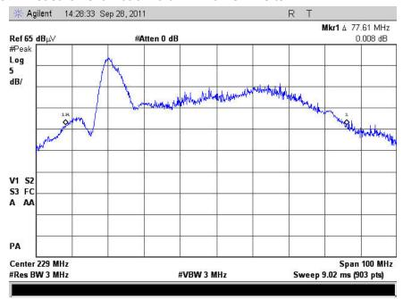
Note: Peak at 199 MHz is channel 11 ambient signal
