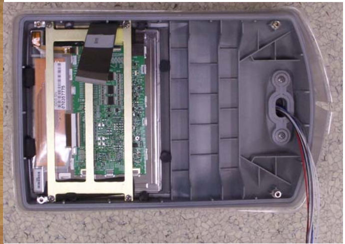
Top mold, bottom side, showing back of display
