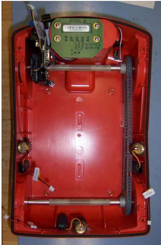
Bottom mold, top side, showing axels, three laser modules and gear belt
