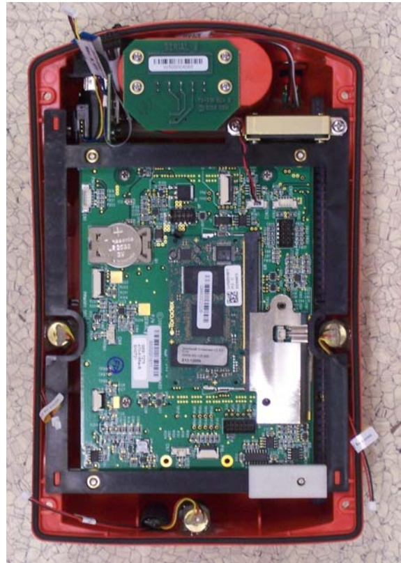
Bottom mold, top side, showing main board installed
