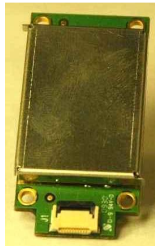
Transmitter with shield attached
