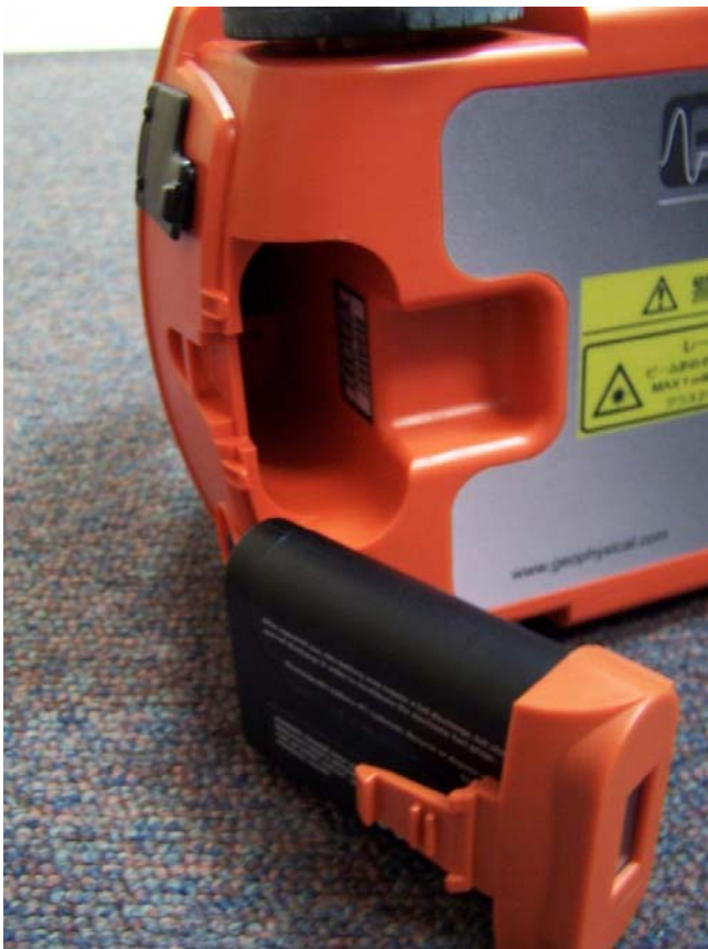
Rear bottom showing battery and battery compartment
