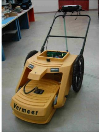
The antenna is constructed as a five-sided metal box, with the antenna fans in the sixth side, on the ground side. The non-transmitting electronics is placed on the top of the shield. Another shield is placed over the electronics.
