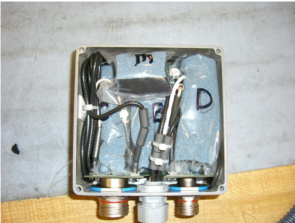
TOP VIEW OF ELECTRONICS WITH BAGGED SHIELDING FOAM
