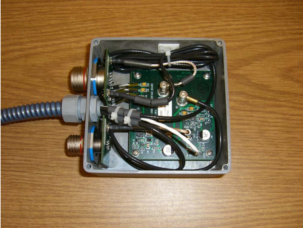
TOP VIEW OF ELECTRONICS WITH BAGGED SHIELDING FOAM REMOVED AMPLIFIER INTERFACE PCB VISIBLE.
