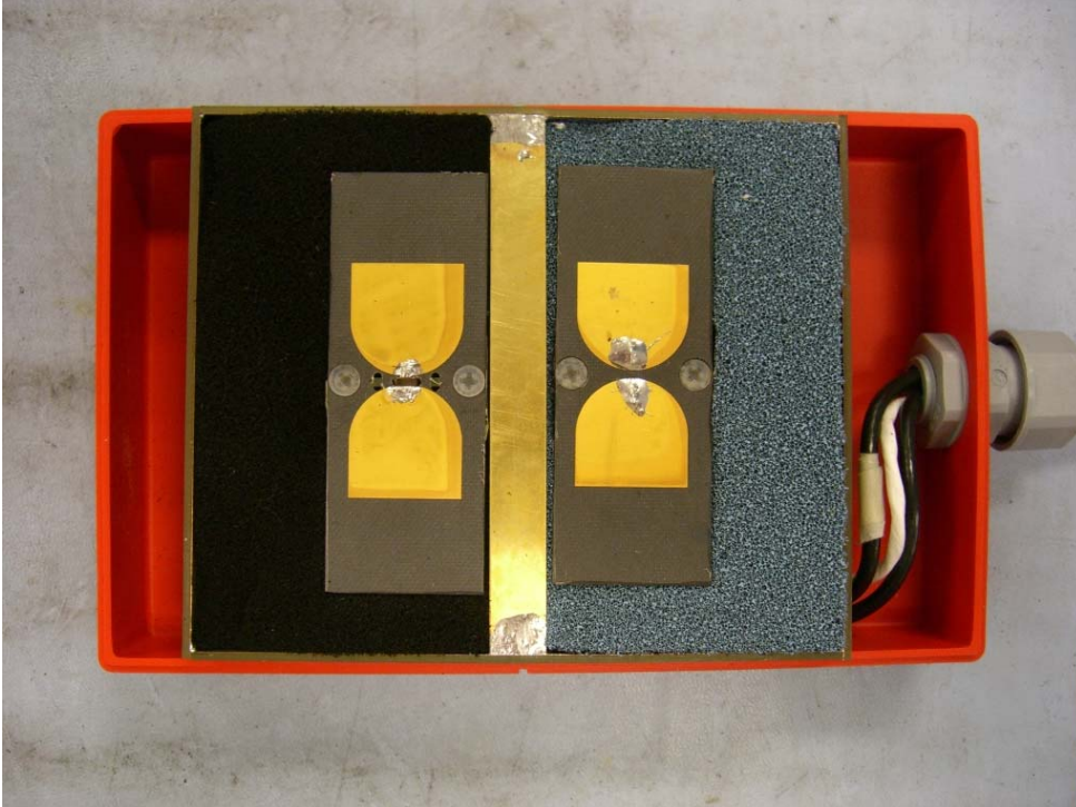
FAN PCB'S AND FOAM PIECES INSTALLED IN SHIELD
