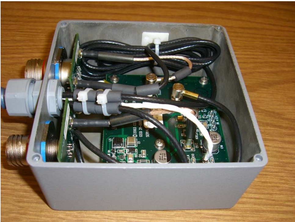
TOP VIEW OF ELECTRONICS SHOWING COILED DELAY LINE
