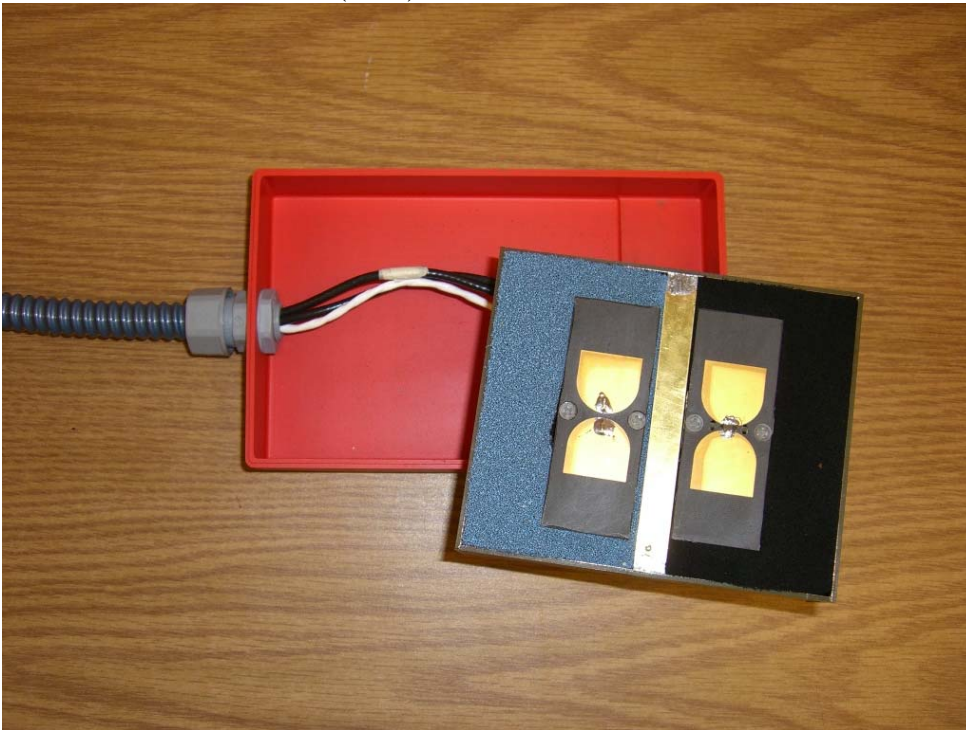
ANTENNA HEAD WITH CASE BOTTOM REMOVED AND TURNED OVER TO EXPOSE FANS.
