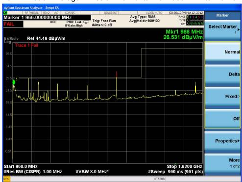
**Note:** Narrow band spike shown over the limit falls under a different rule part / requirement. Cursor is on the peak of the UWB Signal.
