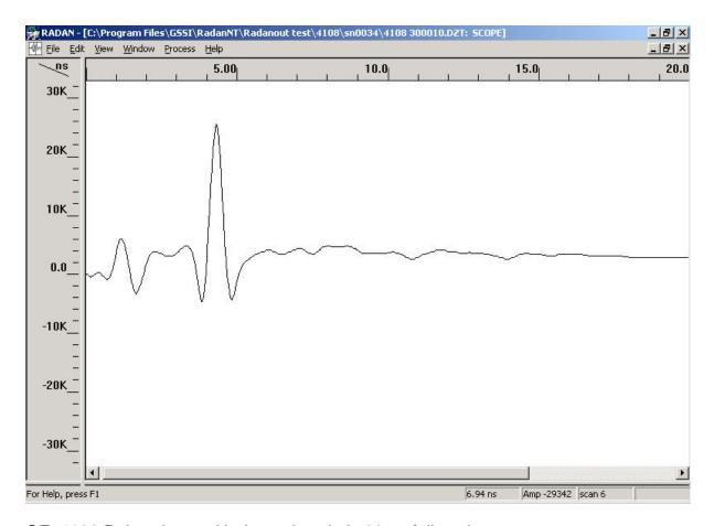
QF74108 Pulse shape. Horizontal scale is 20 ns full scale.
