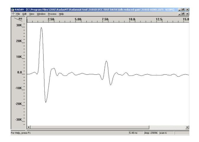
QF73101D pulse shape. Horizontal scale is 15 ns full scale.
