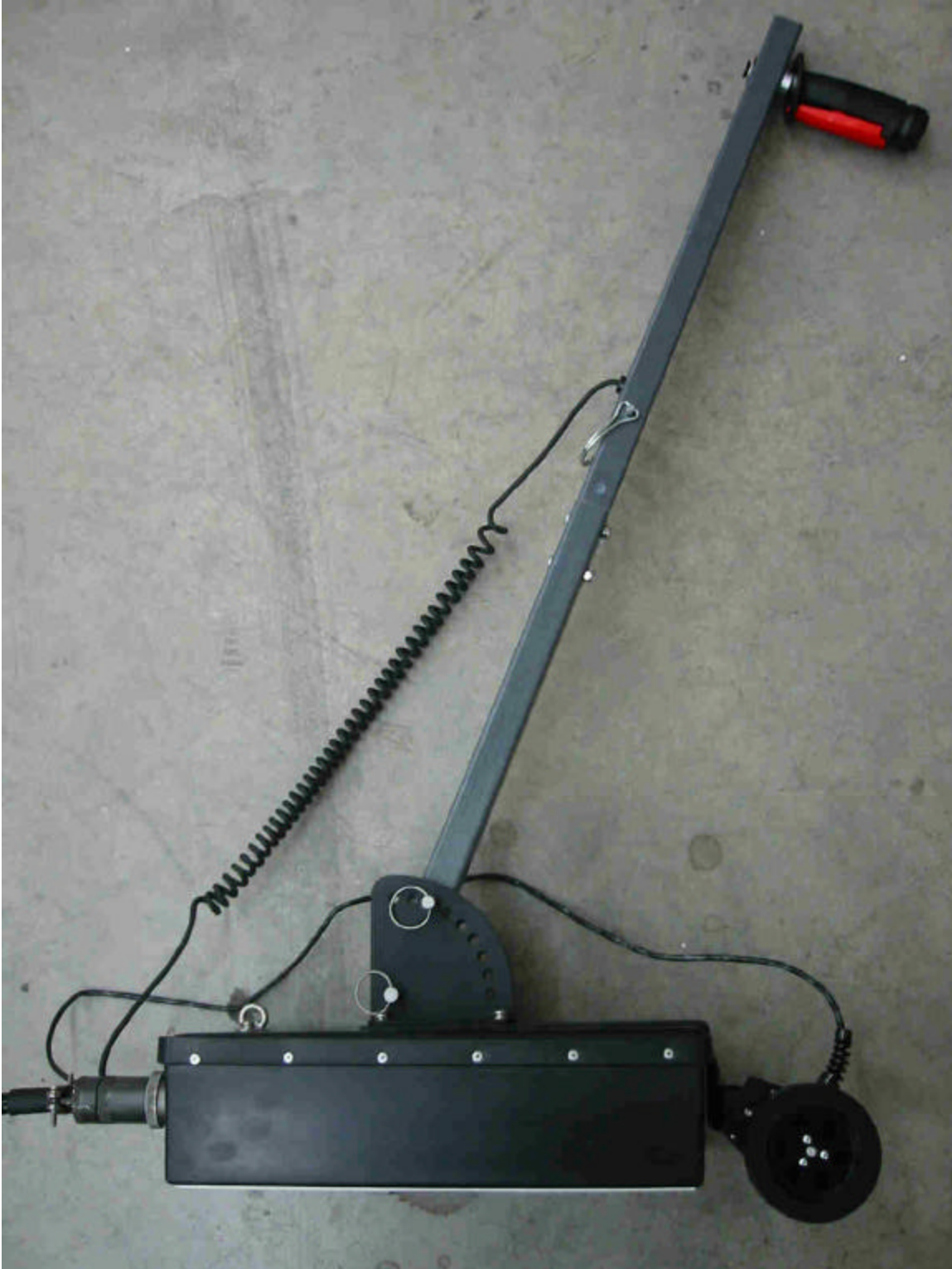
SHOWN WITH MARKER HANDLE, SURVEY WHEEL (FAR RIGHT) AND CONTROL CABLE (FAR LEFT)
