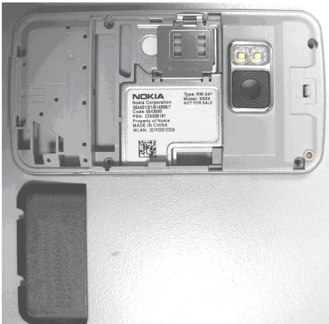
Fig 9 – Rear Housing with Antenna module removed
