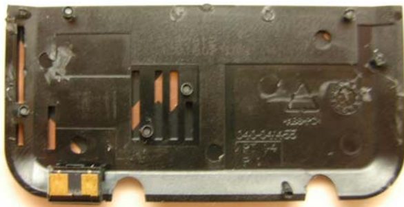
Fig 10 –Antenna module/cover: rear view (Integral 850/900/1800/1900 antennas)
