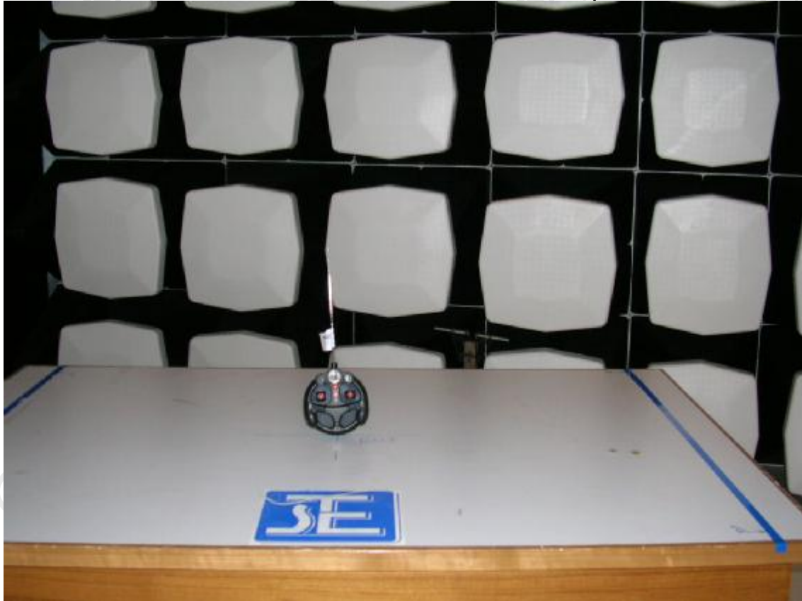
Measurement of Radiated Emission Test Set Up
