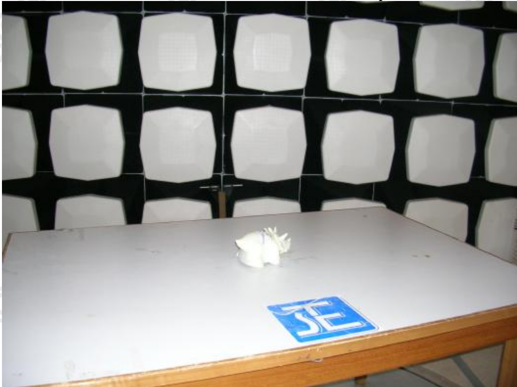
Measurement of Radiated Emission Test Set Up
