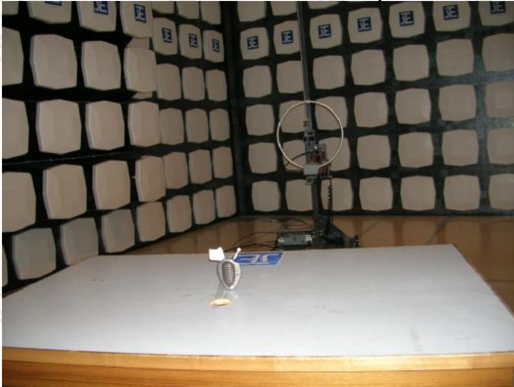
Measurement of Radiated Emission Test Set Up
