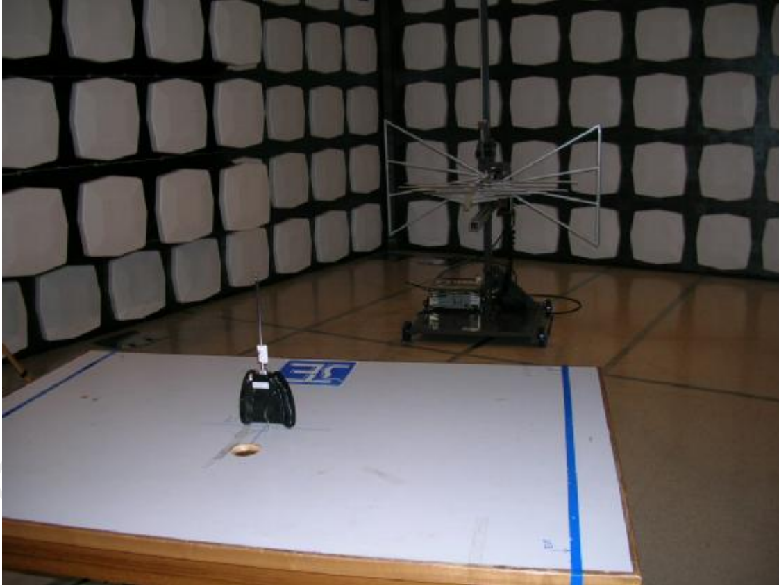
Measurement of Radiated Emission Test Set Up
