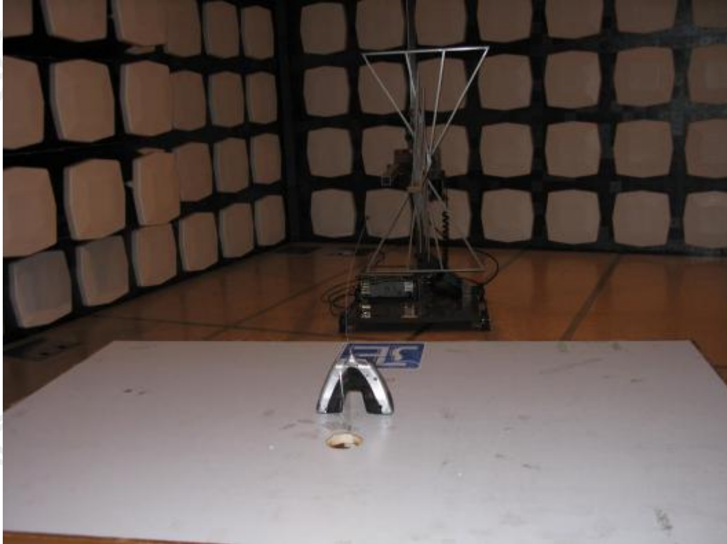
Measurement of Radiated Emission Test Set Up
