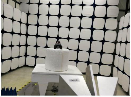
1.3 Radiated Emissions Test Setup
