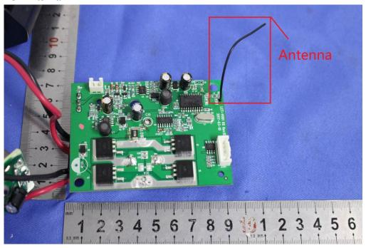
The antenna is integrated on the main PCB and no consideration of replacement. The best case gain of the antenna is 2dBi.
