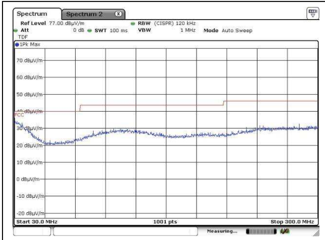
Lower channel, 30MHz – 300MHz, Horizontal
