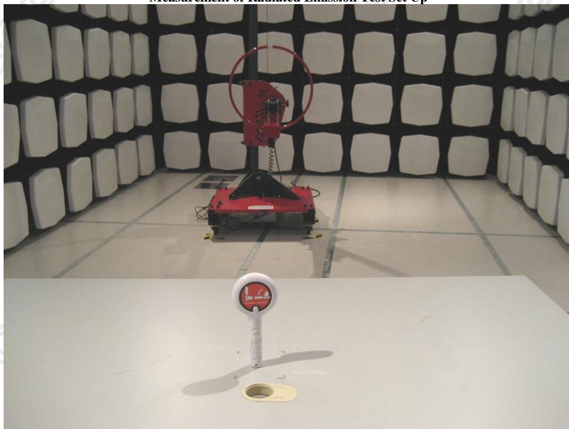
Measurement of Radiated Emission Test Set Up
