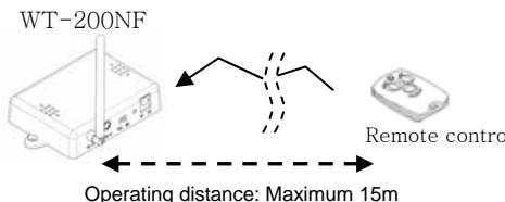
After input operating distance, Emergency signal of special remote control is possible to operate within pre-operated distance
