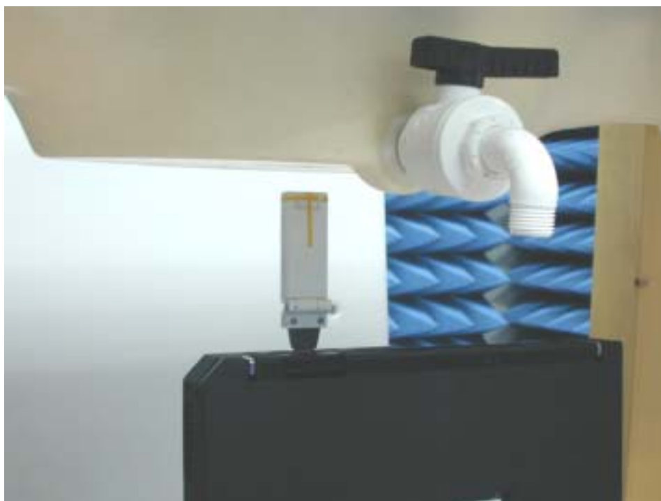
Fig.4 Photograph of the edge of the PC at 90° and at a distance of 1.5 cm from the base of the phantom and the antenna tip upward.
